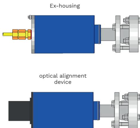
Remove the cover incl. Flame Scanner electronic, replace it with the optical alignment device and fix it with the screws.
