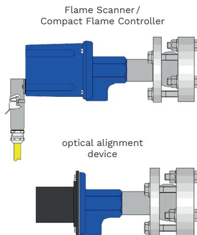
Remove the Flame Scanner / Compact Flame Controller, replace it with the optical alignment device and fix it with the screws.
